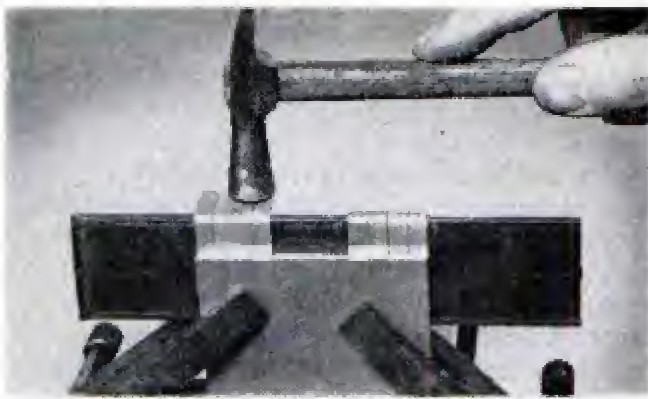
Offset hinge tabs on masks are formed by clamping stack to backing plate and hammering tabs over edge
